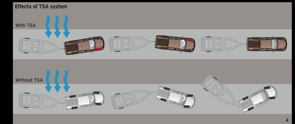
**1.** The 6-airbag system cushions impacts from multiple directions. **2.** DSC automatically controls brakes and traction to help prevent under- or oversteer. **3.** EBA senses emergency braking and boosts brake power. **4.** TSA senses when a trailer begins to sway and varies BT-50's left and right wheel speeds in response.
